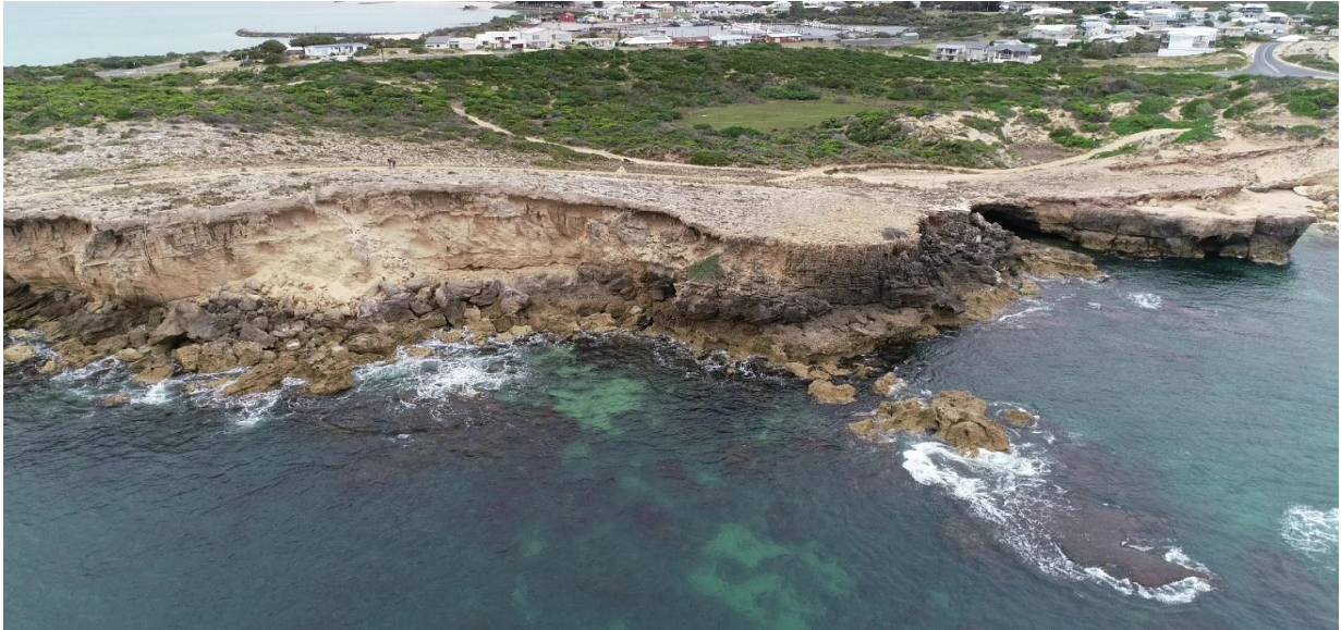
RZ8_0 - Blow Hole Undercutting of Cliff Face- Chainage 1200
