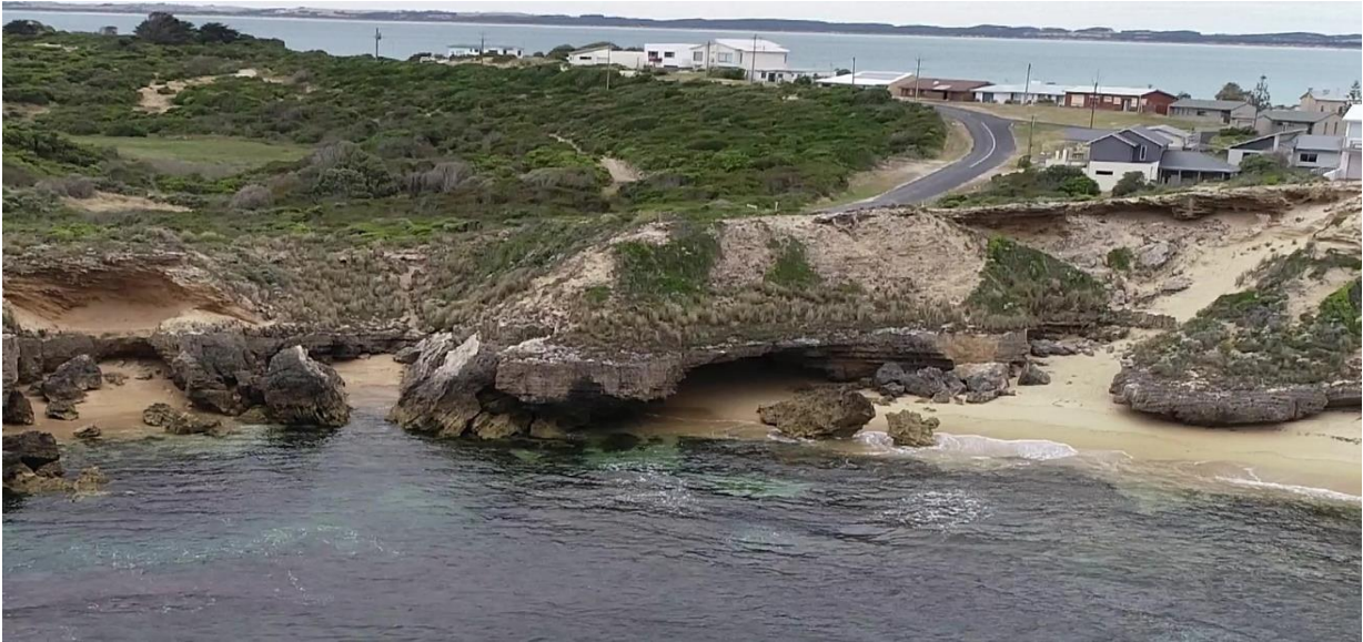
RZ13_0 - Overhanging of Cliff Face - Chainage 1900
