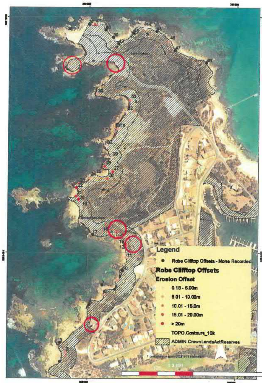
Figure 1 2008 image showing the 48 sites where the cliff top position was compared. Sites are coloured according the extent of erosion (in metres) that was measured. Black indicates no erosion. The red circles show assets located within the 30 metres risk zone - Fotheringham. D, 2009
